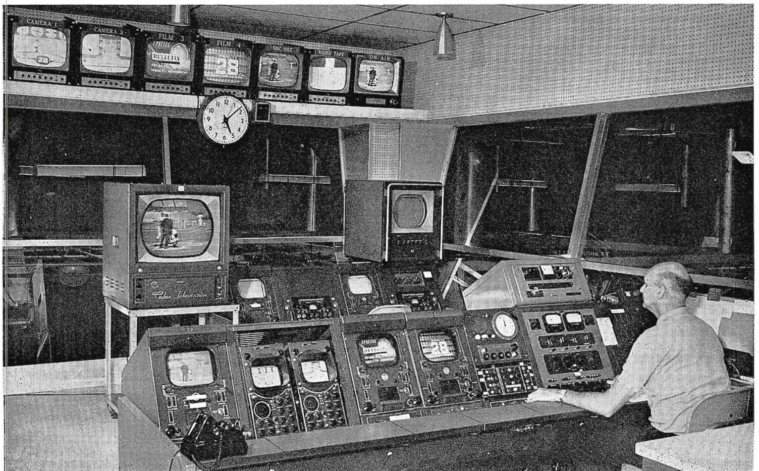
▲ FIG. 12. Two new TR-22 transistorized tv tape recorders, recently installed in the control area. These two compact units are self-contained tv tape recording facilities—require no external racks.
