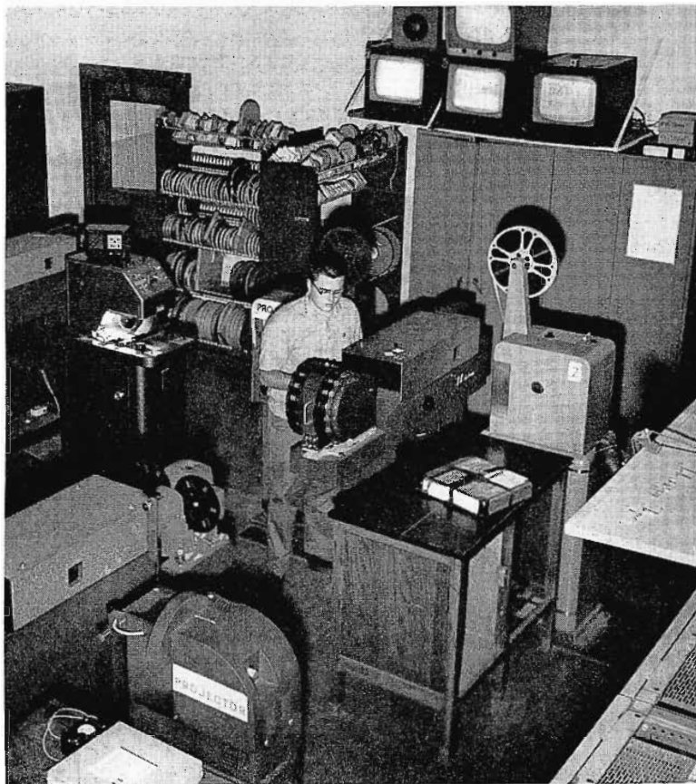
FIG. 11. Projection room, showing three film islands. On 3 monitors in background can be seen Channel 10 and Channel 36 I.D.'s. Film-man John Boeticher loads a slide projector.
