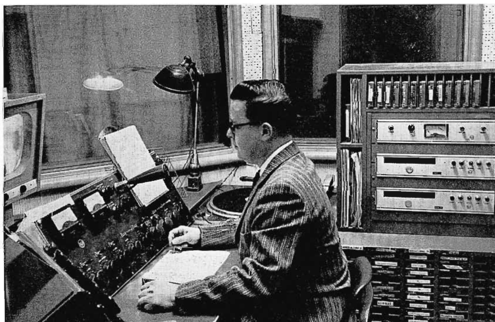
FIG. 15. TV-Audio Control/Announce Booth. Control console is BC-2; 70-D turntable in far corner; BK-1 mike mounted in console. Note two RT-7 Cartridge-Tape Units with recording amplifiers at far right. George Hack awaits a video cue.
